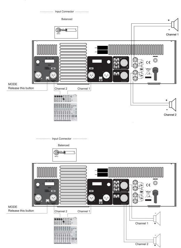
You can also operate the paralleled mode via outside wiring, so, the signal input from channel 1 or 2 will be output from both channel 1 and 2 simultaneously. The volume of channel 1 or channel 2 can be controlled separately.
